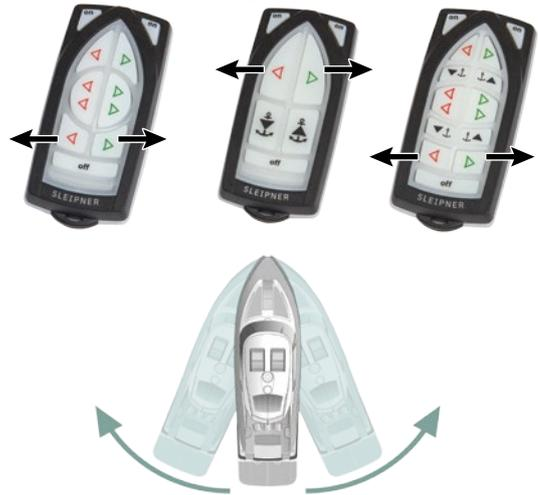
Activating both bow and stern thruster to push the boat sideways
